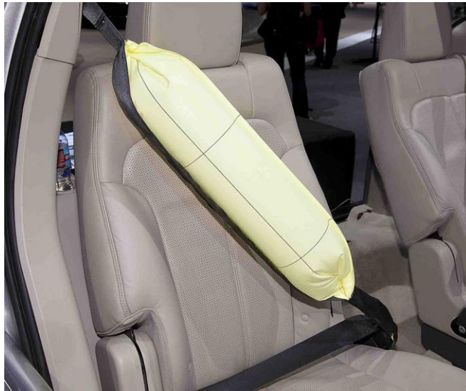
Fig. 5. Inflatable seat belts
