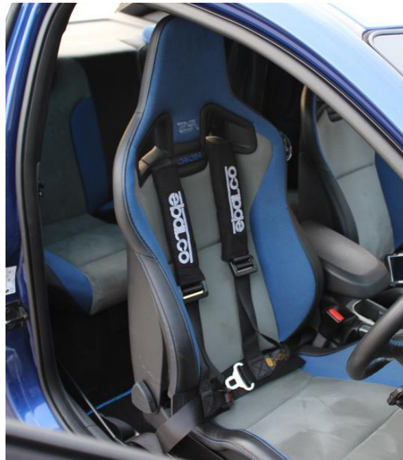
Fig. 3. Four-point seat belt
