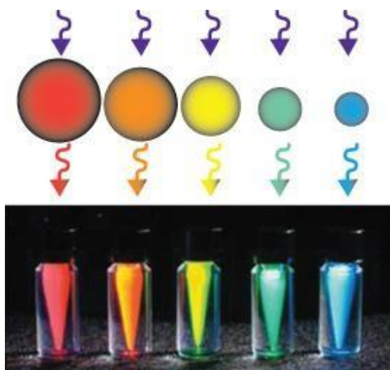
Figure 5. The color of quantum dots depends on their size
